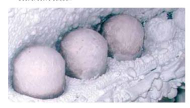
Interchar Bolt Caps retain material integrity during and after fire exposure thus protecting the underlying bolt connections against embrittlement caused by rapid quenching from firefighters hose stream.
